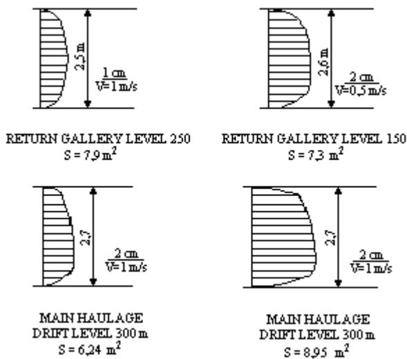
Fig. 1. Air velocity profiles in TH – arch supported mine workings, Petrla Colliery
