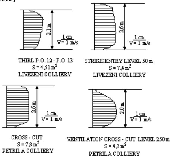
Fig. 2. Air velocity profiles in concrete supported mine workings, Livezeni and Petrla Collieries
