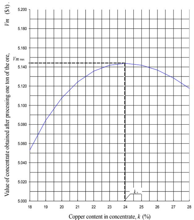
Equation (8) shows that the optimal copper content in concentrate does not depend on the copper content in the ore ( $u$ ).
