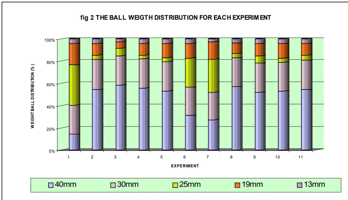
From point of view of weight composition, presented in figure 2, is seen a reduced quantity of small balls comparative with coarse balls, the average classes being representative in experiments 1, 6 and 7. In all other experiments, balls with diameter value of 40mm represent higher than 50% in charge weight.
