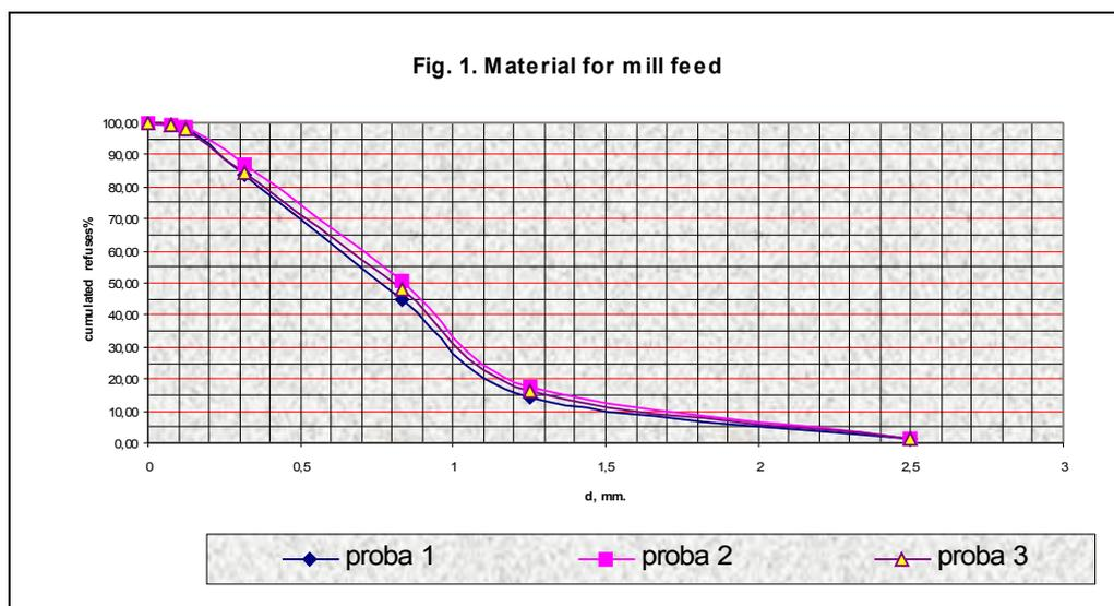
The samples were tested complying with a pre-established program, following all the stages of the test. The program refers to establish the influence of size ball charge, like average size, on Bond index value. In this experiments, the feed sized, the ball charge and the mill revolution were unchanged.
