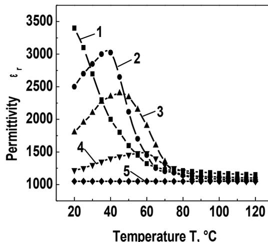
Fig. 4. Dependence of the dielectric permittivity  $\epsilon_r$  on the concentration of the  $\text{MgZrO}_3$  calcinated at a temperature of  $1400^\circ\text{C}$ ; 1)  $x=0.15$  mol; 2)  $x=0.20$  mol; 3)  $x=0.25$  mol; 4)  $x=0.30$  mol; 5)  $x=0.35$  mol
