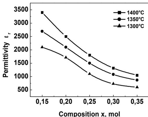
Fig. 1. Dependence of the dielectric permittivity  $\epsilon_r$  of the materials on the concentration of  $\text{MgZrO}_3$  and calcination temperature
