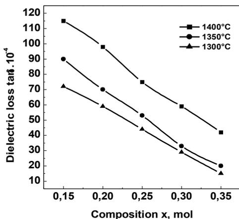
Fig. 2. Dependence of the dielectric losses  $\tan \delta$  of the materials on the concentration of  $\text{MgZrO}_3$  and calcination temperature
