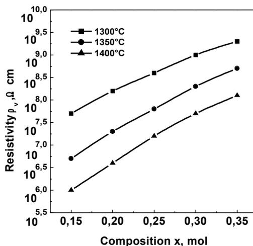
Fig. 3. Dependence of the resistivity  $\rho_v$  of materials on the concentration of  $\text{MgZrO}_3$  and calcination temperature
