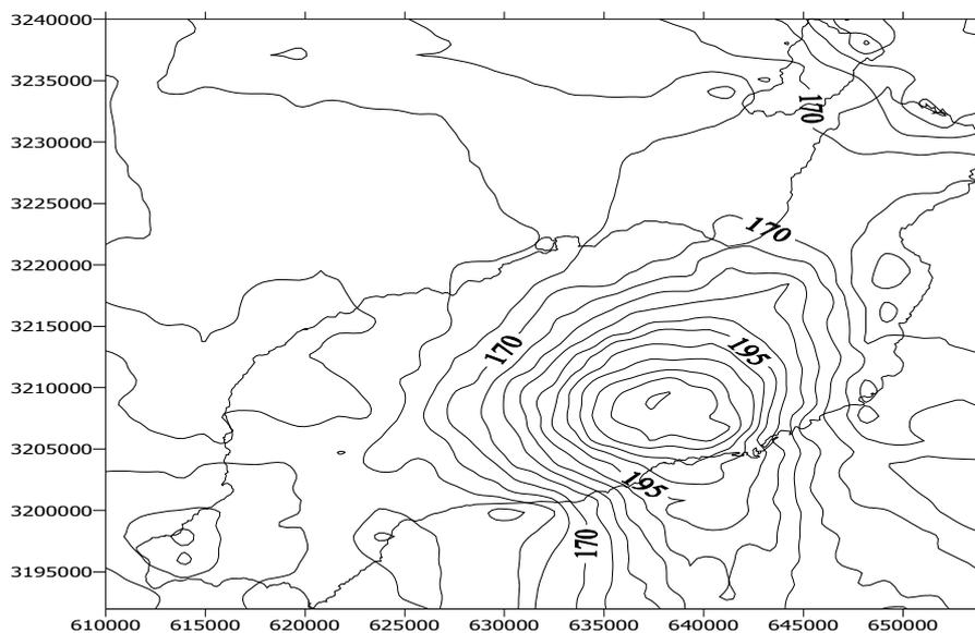
Fig. 2. Refined Bouguer anomaly observed. Contour interval 5 m Gal, coordinates in meters. Besides the lines of the observations, the boundaries of the islands are also given
