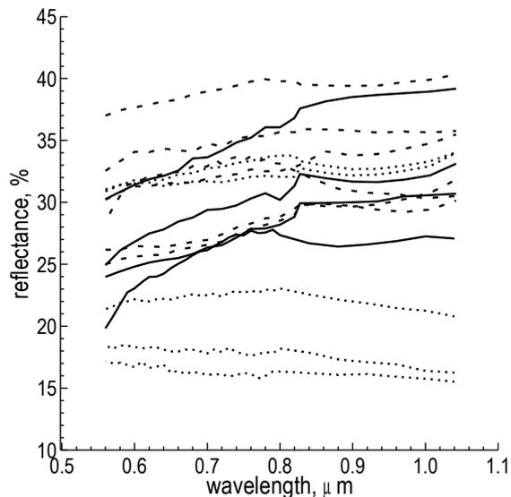
Fig. 1. Spectral reflectance of granites
