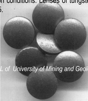
Figure 5. Working media of tungsten carbide
