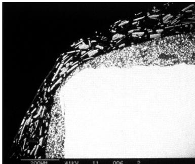
Figure 4. Cross-section of covering of MIO.
