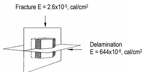
Figure 2. Needed energy for destruction of hematite crystal
