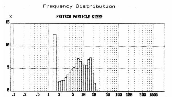
Figure 6. Granulometric characteristic of hematite.
