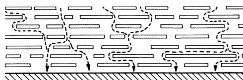
Figure 3. Barrier effect created by MIO particles
