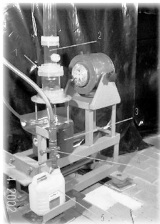
Figure 4. Vibratory column flotation machine – basic parts
