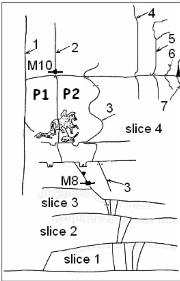
Fig. 4. The main cracks (1-7), slices (1-4), rock prisms (P1 and P2), and monitoring sites (M8 and M10) at the rock monument
