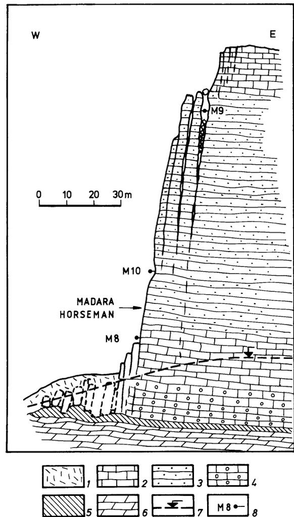
Fig. 3. Engineered-geological profile of the Madara Plateau (modified after Frangov et al., 1992): 1 – slope deposits; 2 – whitish sandy limestone; 3 – yellowish calcareous sandstone; 4 – conglomerated limestone; 5 – yellow montmorillonite clay; 6 – grey marl; 7 – groundwater table; 8 – extensometer for 3D monitoring
