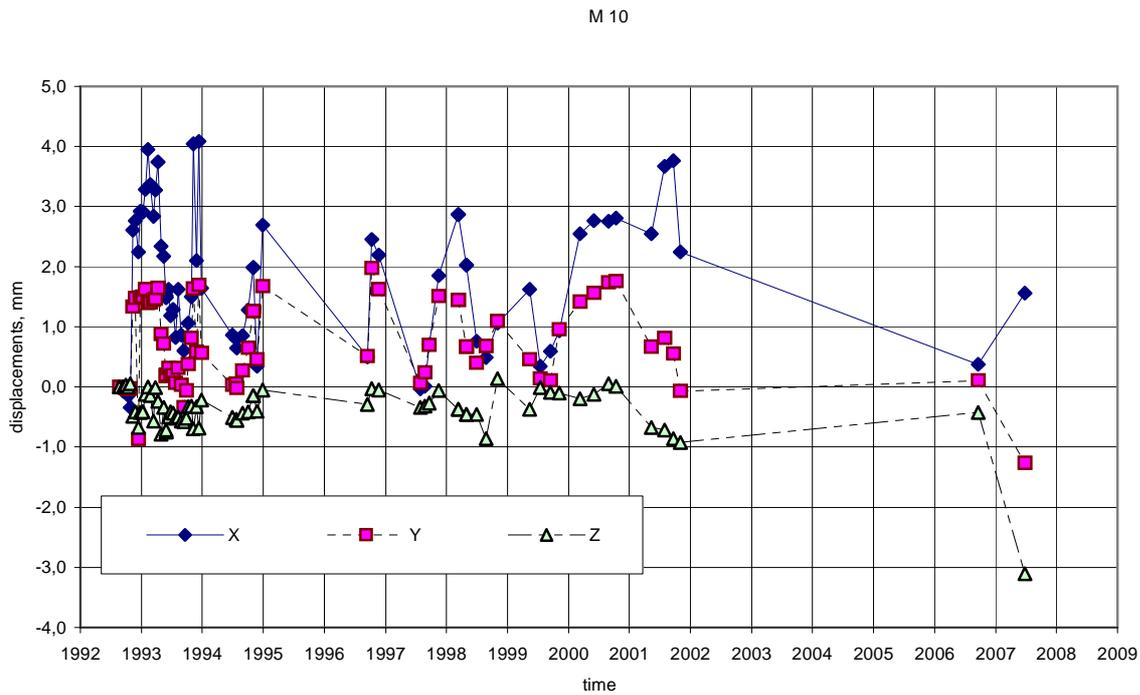
Fig. 7. Diagram of displacements established at monitoring point M10 for the period 1993-2008: +X – extension of the crack; +Y – moving of the rock prism P2 inside the massif; +Z – uprising of the rock prism
