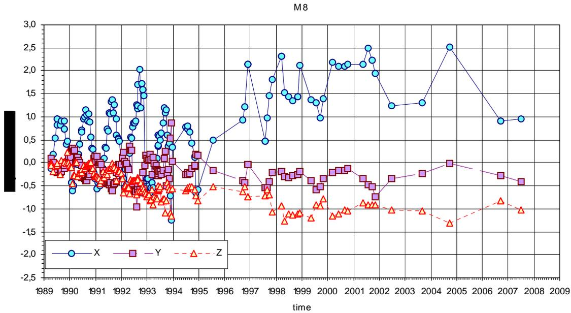
Fig. 6. Diagram of displacements established at monitoring point M8 for the period 1990-2008: +X – compression of the crack; +Y – moving of the rock prism P2 inside the massif; +Z – uprising of the rock prism
