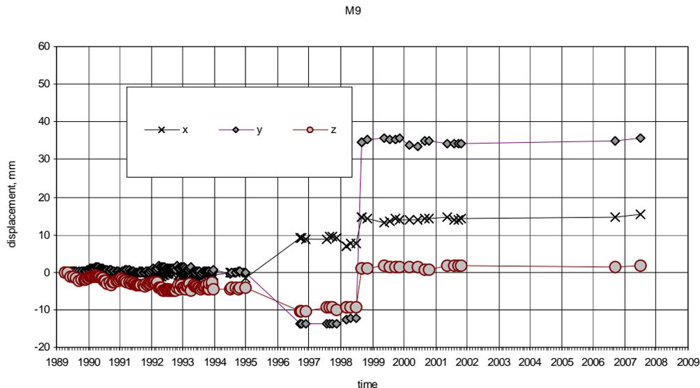
Fig. 5. Diagram of displacements established at monitoring point M9 for the period 1990-2008: +X – compression of the crack; +Y – the rock slice to SSE; +Z – uprising of the rock slice
