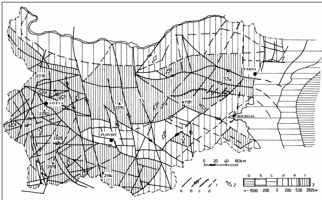
Fig. 1. Scheme for the general block fragmentation and the horizontal and vertical block movements in Bulgaria: 1 – fault and photolineament: a – well noted fault and photolineament, b – strike-slip fault, c – reverse fault and nappe lines, d – unsurely noted fault and photolineament, 2 – direction of horizontal block movement, 3 – vertical movements in indicated intervals of height
