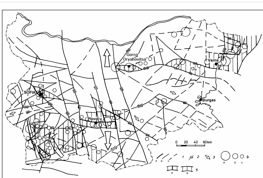
Fig. 2. Earthquake epicentre distribution in the country: 1 – fault and photolineament, a – very well noted one, b – well noted one, c – unsurely noted one; 2 – strike-slip fault; 3 – direction of horizontal block movement; 4 – earthquake with following magnitudes M, a –  $M \geq 7.0$ , b –  $M = 5.0-6.9$ , c –  $M = 3.0-4.9$ ; 5 – blocks with significant concentration of epicentres, a – with biggest one, b – with big one
