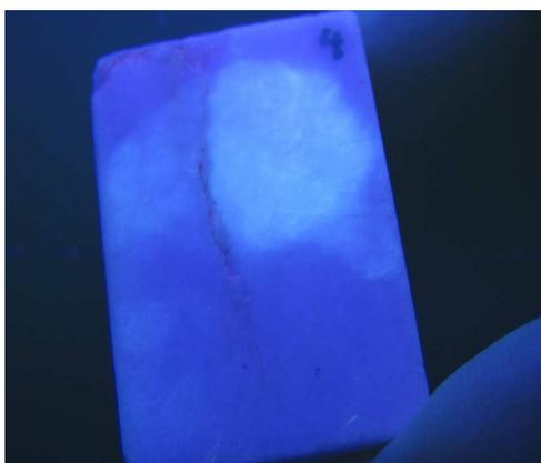
Fig. 1. Frustumation character within the Karrara (Toskana, Italy) calcite-dolomitic statuary marble revealed under UV-irradiation. Two types of frustums due to UV-luminescence of oxygen defect complexes: light-blue and dark-violet with the maximum about 490 nm wave length strip (Gotze et al., 1999); length of the sample short edge – 3 cm
