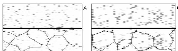
Fig. 2. Frustumation supertexture pattern of rocks inner composition visualised with the help of laser ultrasonic echoscopy: A – medium-fine grained Kibik-Kordonsky calcite-dolomitic marble, B - medium-fine grained Kyshtymsky granulated quartzite. Specimen width: 13 and 12 mm, relatively. Upper part of picture – original pattern, lower – retouched
